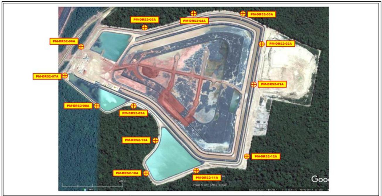
Figure 4.23 Monitoring wells at DRS2
