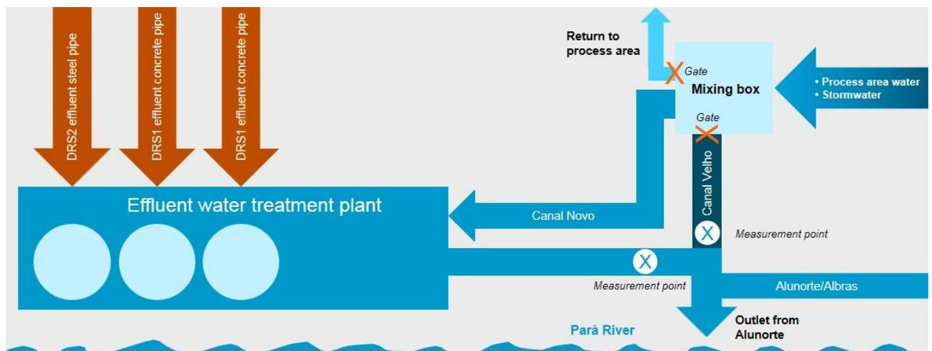
Figure 4.16 Principle of effluent treatment plant at Alunorte
