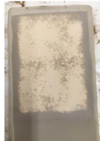
Picture 3: Example test panel, system DFT: 2 x 100µm (4 mils) of Epoxy Phenolic. The topcoat has been eroded to show the primer coat below.
