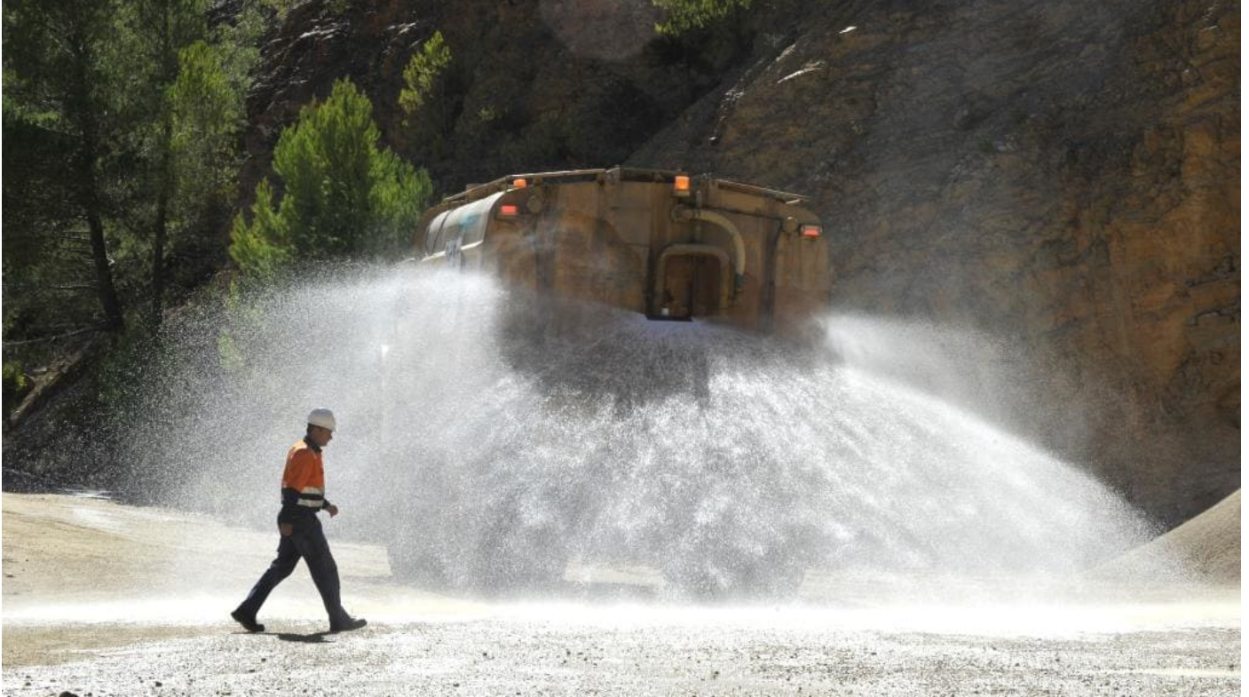
Figure 2 A safety inspector at a Stonyfell quarry with a truck spraying water to dampen the dust in 2011.
