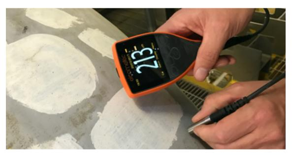
Measuring Dry Film Thickness (DFT) of an Epoxy Phenolic Coating (Source: ExcelPlas)
