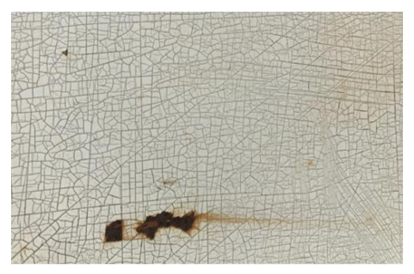
Mosaic Cracking and Underlying Corrosion of an Epoxy Coating on a Metal Tank (Source: ExcelPlas)
