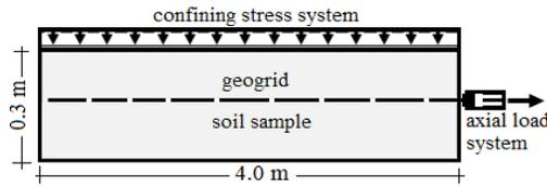
Fig. 1. Pull-out test device.
