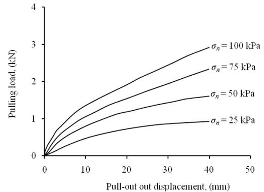
Fig. 2. Load-displacement relationships of the geogrid.
