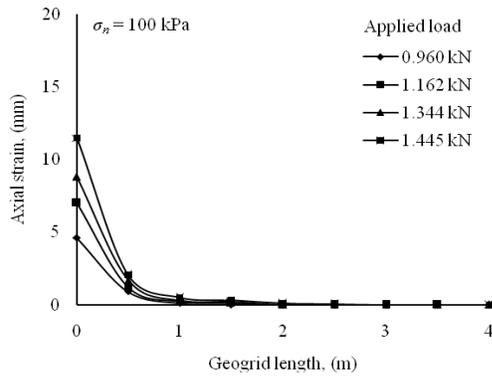
Fig. 3. Axial deformation along the geogrid.
