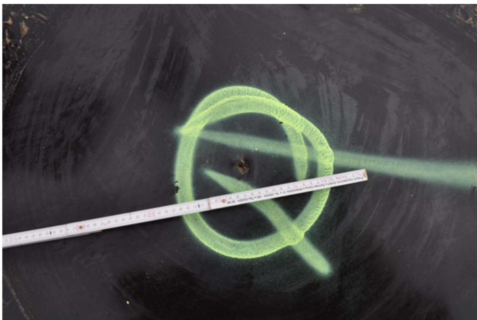
Figure 4. Defect caused by a pointed object found in the HDPE GM of landfill 'Da'
