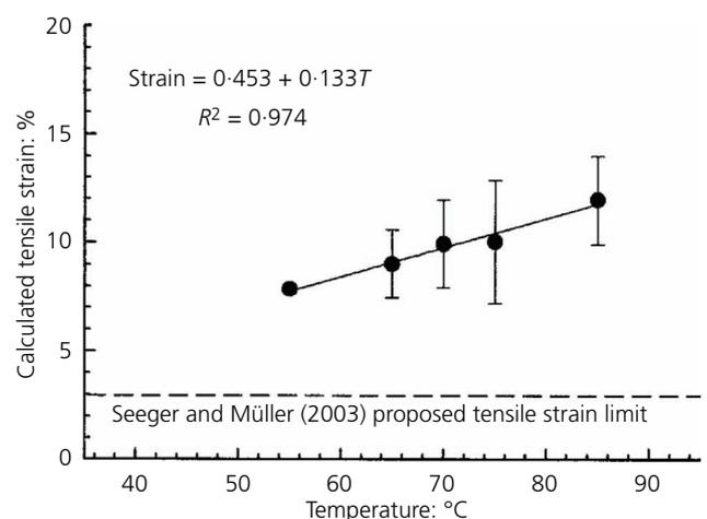
**Figure 6.** Maximum strain in the outer fibre of the GM, at which stress crack formation was observed, as a function of test temperature. The data were taken from Abdelaal *et al.* (2014)
