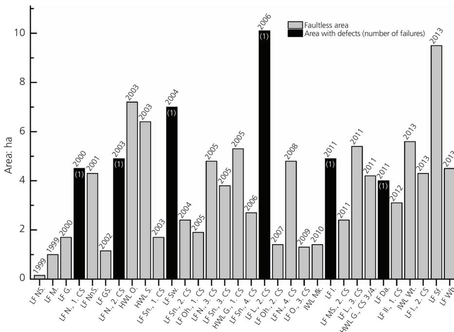
Figure 3. Monitored areas of capping systems with LDSs of anonymised landfills in Germany. The year of construction is indicated above and the number of failures within the bars. LF, landfill; HWL, hazardous waste landfill; IWL, industrial waste landfill; CS, construction section
