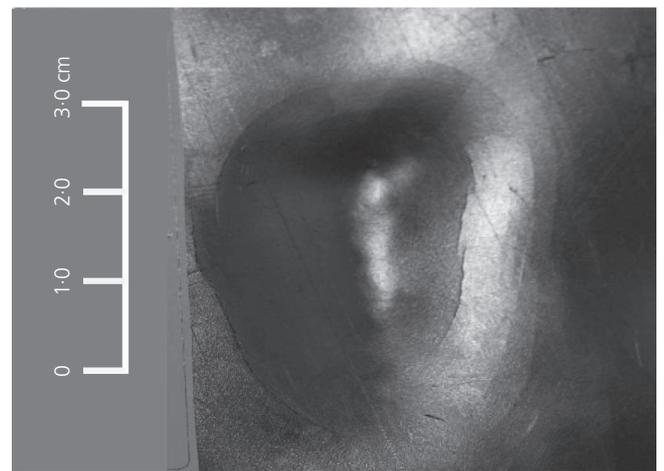
**Figure 5.** Stress crack formation at the edge of indentation as formed during a long-term load test at 75°C with a pre-aged 1.5 mm thick HDPE GM protected by a 560 g/m<sup>2</sup> non-woven geotextile PL against coarse gravel ( $D_{10} = 32$  mm,  $D_{85} = 55$  mm, particle diameters at which 10% and 85% by weight of the particles are finer). The picture is from Abdelaal *et al.* (2014) reproduced with permission of the publisher
