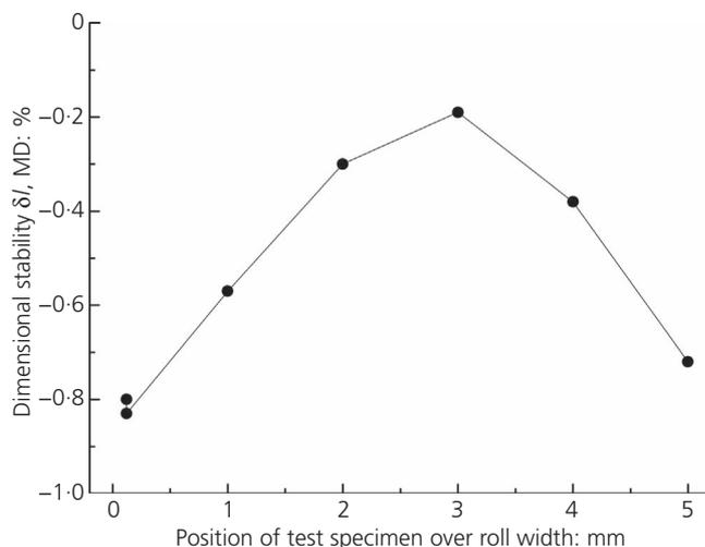
Figure 1. Dimensional stability (MD, machine (extrusion) direction) along the width of GM
