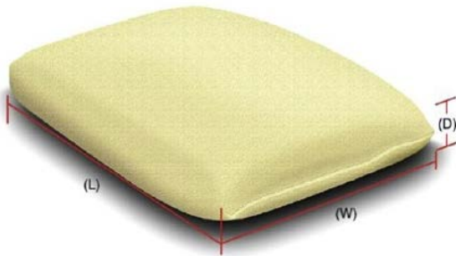
Figure 1 Geotextile bag dimensions (Source: [5]).
