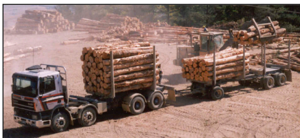
Figure 3. A commonly configured on-highway 7-axle log truck being loaded at a landing.
