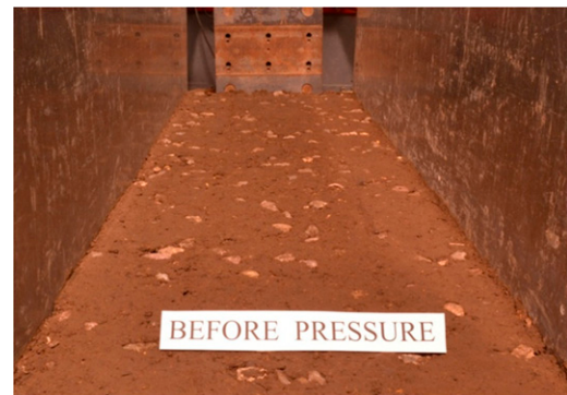
Fig. 4. Surface of gravelly CCL after compaction for Test 5H1
