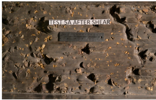
Fig. 12. CCL surface after shearing stage for GM/CCL Test 5A (shear direction is to the right)
