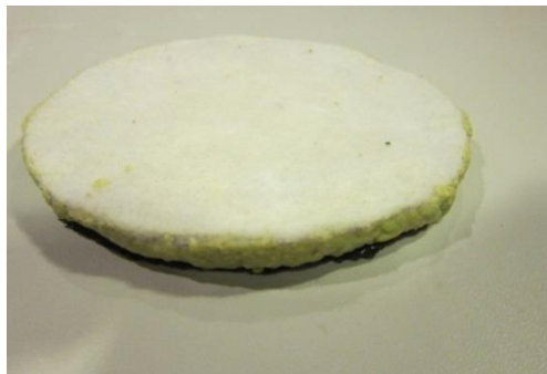
Fig. 10. GCL Specimen having 100 mm Diameter (Nonwoven Side Up)
