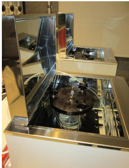
Fig. 12. Permeameter Cells in Water Tanks
