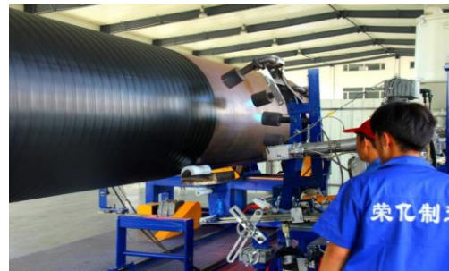
Heating device of the first station of production line of PE large-diameter long fiber reinforced composite feed/drain pipe
