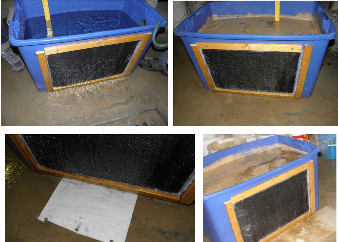
Figure 7. Woven slit film geotextile simplified filtration test
