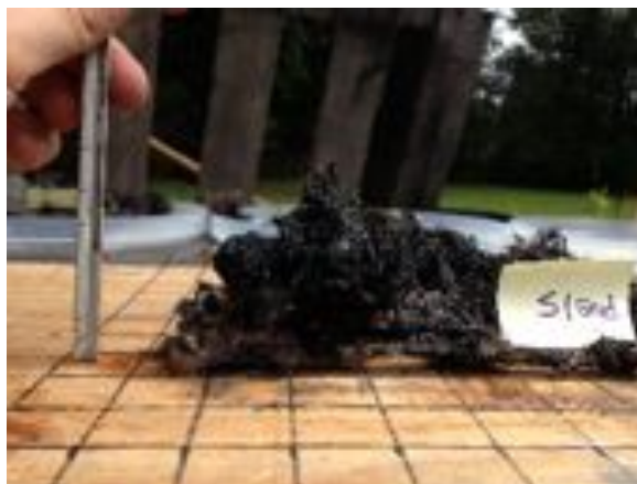
Figure 6. Example Material Growth Observed from the Side
