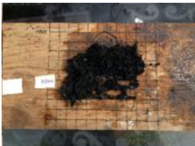
Figure 7. Example Wet Growth on Substrate Sample on 1" by 1" grid for Area
