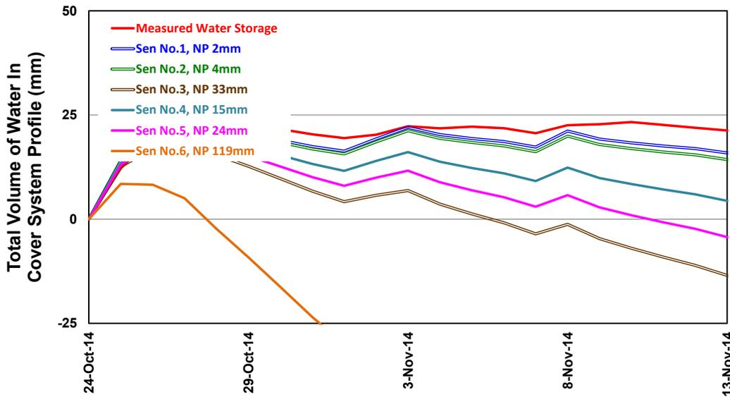
Figure 9. Calculated change in water storage in the cover profile using simulated net percolation from Scenario No.1 through No.6.
