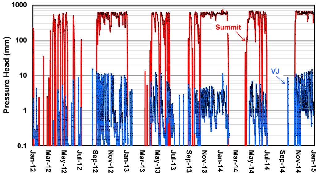
Figure 4. Hydraulic head above the geomembrane at Summit and VJ over the 2012 to 2014 monitoring period.
