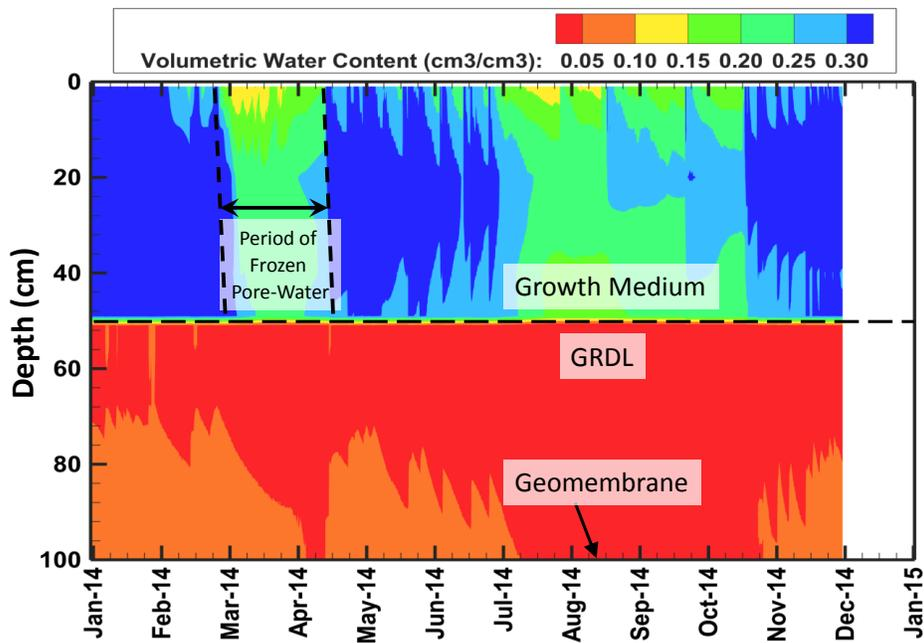
Figure 2. 1-D isopleth contour of the VJ cover system volumetric water content profile depicting adequate lateral drainage capacity in the GRDL. Note: ‘drying’ in the growth medium layer in the winter (i.e. February and March) is artificial and is due to a change in the dielectric constant of pore-water when it freezes.
