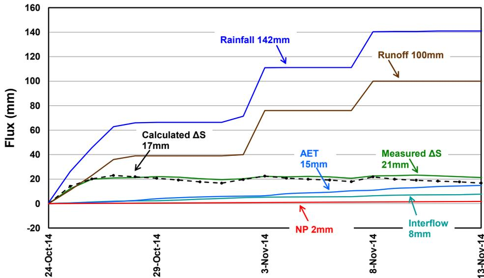
Figure 8. Water balance for the reclaimed Summit WRP and the calculated change in water storage using Scenario No. 1 (net percolation 2 mm in the period).
