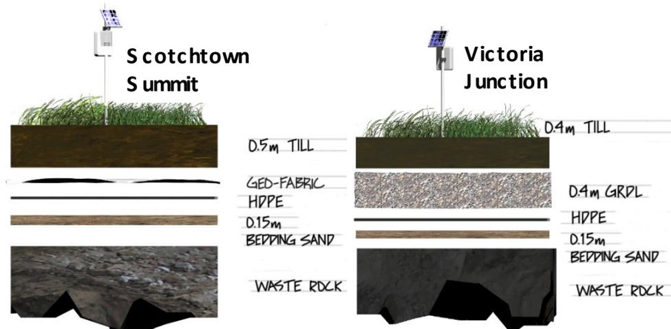
Figure 1. Schematic of the Summit and VJ WRP cover systems.
