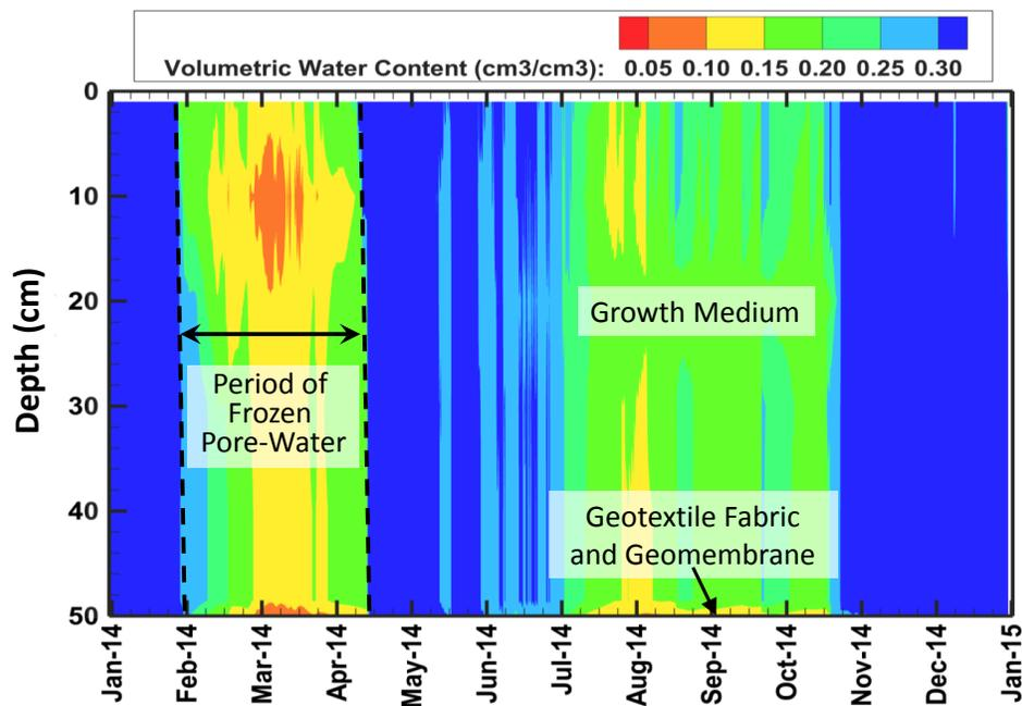
Figure 3. 1-D isopleth contour of the Summit cover system volumetric water content profile depicting limited lateral drainage capacity in the growth medium. Note: ‘drying’ of the growth medium layer in the winter (i.e. February and March) is artificial and is due to a change in the dielectric constant of pore-water when it freezes.
