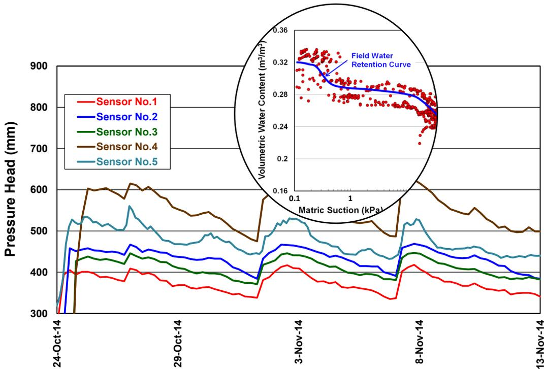
Figure 10. Pressure head measure in transect across cover system profile along with inset figure of field water retention curve based on monitored volumetric water content and suction.
