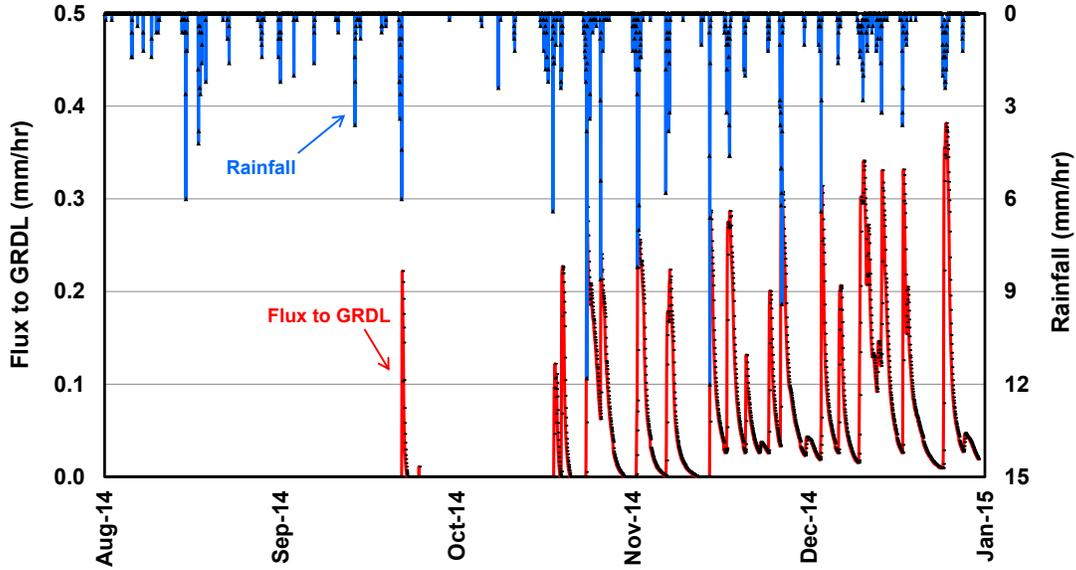
Figure 5. Rainfall and water ingress to the GRDL for the JV cover system.
