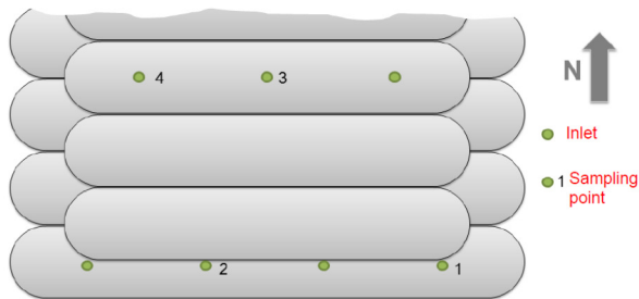
Figure 5 Location of the inlets and sampling points of the analysed tubes at the Southern corner of the first dewatering field
