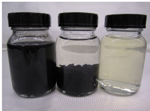
Figure 1 Effect of blending polymers and effluent water after filtration with high performance filter fabric (from left to right: original sludge; “flocculated” sludge, blended with appropriate polymer; filtrate)
