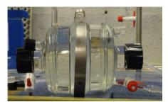
Figure 1: dual cell permeameter (overview)
