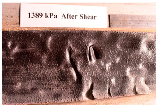
Fig. 17. Geomembrane for DL/GT/GM/S Test P10 after shearing stage
