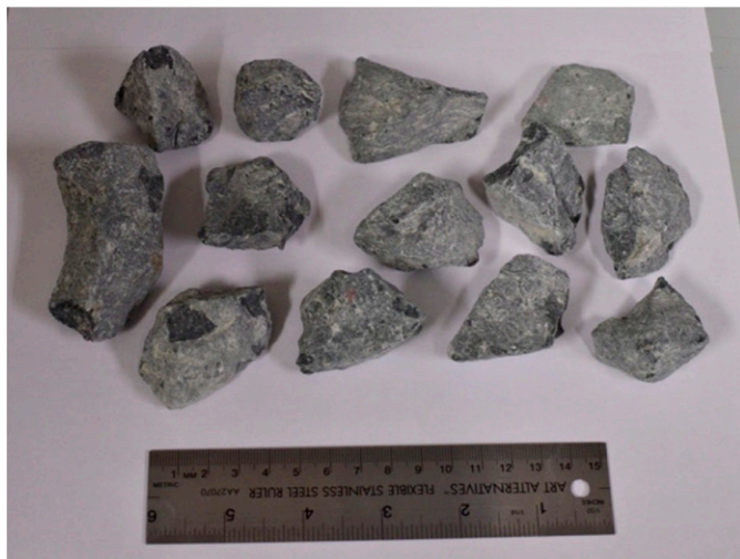
Fig. 2. Gravel particles for drainage layer (scale length = 152.4 mm)
