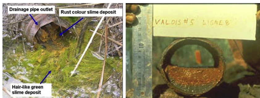
Fig. 5. Ochre deposits around drainage pipes and filters. After Mendonca and Ehrlich, 2008.
